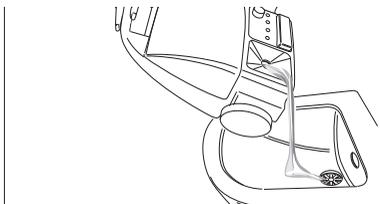
Rinse the boiler of the steam cleaner boiler at the latest after 5 boiler fillings.
