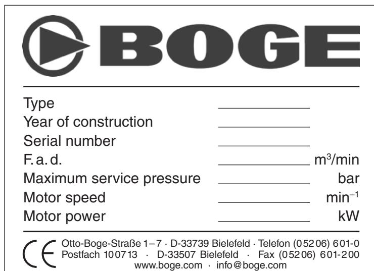
Fig. 1.1: Data on the type plate
