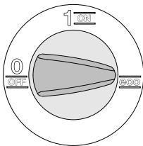
There are the switch positions "1/ON" and "eco" to switch the appliance on.
