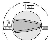
There are the switch positions "1/ON" and "eco" to switch the appliance on.
