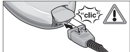
Figure 1: Inserting the modular accessory plug
