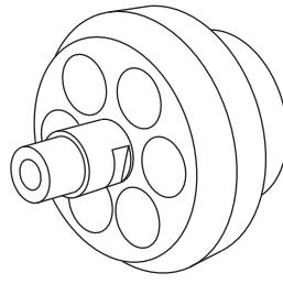
The working light is connected between the jet pistol and the nozzle. Switching on and switching off is described in the chapter "Operation/Basic Settings".
