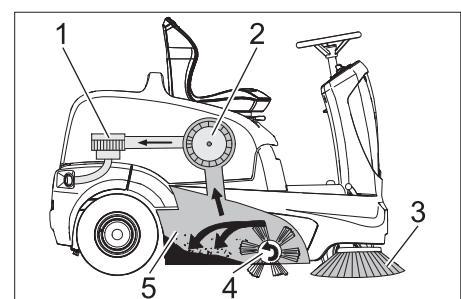
The sweeper operates using the overthrow principle.
