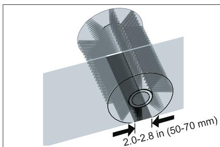
The sweeping track should have an even rectangular shape which is between 2.0 and 2.8 in (50 and 70 mm) wide.
