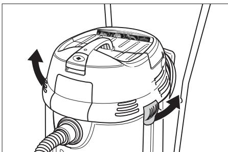
→ Release and remove the vacuum head.
