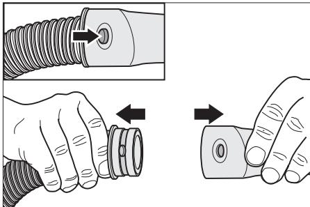
The suction hose is equipped with a clip system. All C-40/C-DN-40 accessories can be connected.
