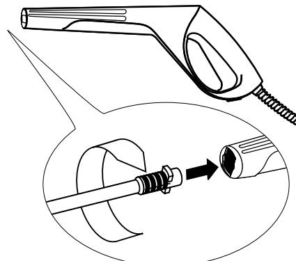
**Step 2** Insert the spray wand of your choice into the trigger gun. Push in and turn clockwise to lock spray wand in place.
