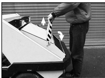
Lift and close container ejection tailgate
