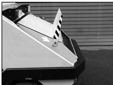
The container debris ejection door must lock in place.
