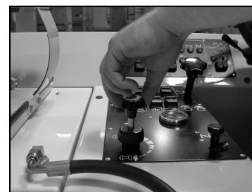
Motor speed: Fine adjustment
