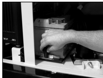
Unscrew the battery holder Take out the battery by the lifting loops
