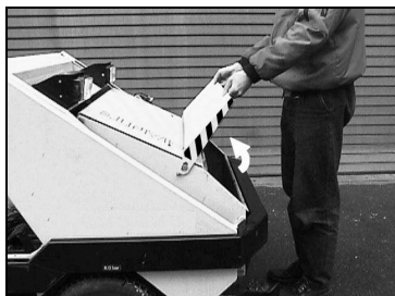
Legingsklep reservoir openen
