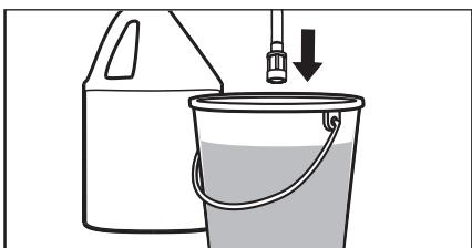
**Step 2** Fill the detergent reservoir with Kärcher detergent. Place the filter end of detergent suction tube into the detergent reservoir
