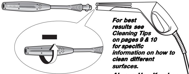
**Step 1** Install the Vario spray wand. Set the Vario spray wand to the low pressure setting (-) by turning the wand collar. The wand must be set in the low pressure (-) position to apply detergents.
