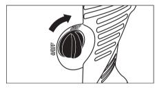
**Step 6** Turn on the pressure washer. The motor starts only if the trigger of the gun is pulled and shuts off when the trigger is released.
