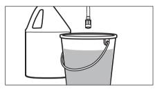
Step 2 Fill a container with Kärcher detergent. Place the filter end of detergent suction tube into the container.
