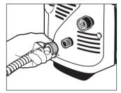
**Step 6** Disconnect the high pressure hose from the high pressure outlet.
