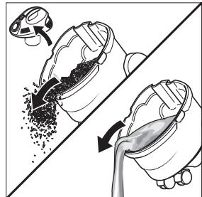
**Clean filter by holding the filter under running water.**
