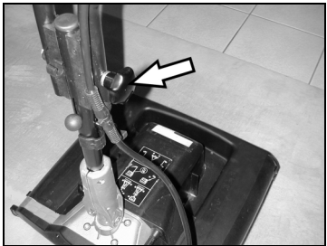
Adjust the upper half of the pushing handle and fix it with the knurled screw
