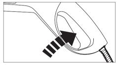
**Step 5** Plug the power cord into the power outlet. Unlock the lock of the trigger gun. Trigger the gun to eliminate trapped air, wait for a steady flow of water to emerge from the spray nozzle.
