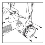
**Step 1** Slide each of the mobile adapter brackets to the pressure washer. Align the pegs and holes on the brackets. Insert the 4 screws and tighten as shown.
