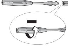
**Step 1** Install the Wash Brush or Vario spray wand. Set the Vario spray wand to the low pressure setting (-) by turning the wand collar. The wand must be set in the low pressure (-) position to apply detergents.
