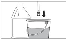
**Step 2** Fill the detergent reservoir with Kärcher detergent. Place the filter end of detergent suction tube into the detergent reservoir
