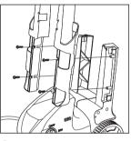
**Step 2** Slide the handle onto the mobile adapter brackets as shown, insert screws and tighten.
