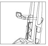
**Step 3** Slide the hose caddy into the handle slots and snap into place.
