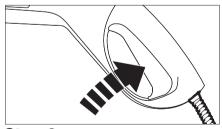
**Step 3** Turn on the pressure washer. Pull trigger to operate unit: Liquid detergent is drawn into the unit and mixed with water. Apply detergent to work area. Do not allow detergent to dry on surface For best results see Cleaning Tips on pages 9 & 10 for specific information on how to clean different surfaces.
