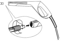
**Step 4** Pull out the locking slide from the right side of the trigger gun handle, and insert the small end of the high pressure hose into place. Push the locking slide back into the trigger gun to lock the hose in position.
