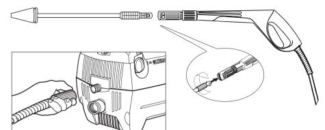
Step 1 Connect the high pressure hose to the unit's high pressure outlet. Step 2 choice int
