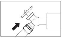
**Step 4** Connect garden hose to the cold water source and turn water on completely.
