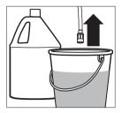
**Step 1** Remove detergent suction tube from container and insert into 1 gallon of fresh water. Siphon water at low pressure for one minute.
