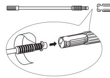
**Step 1** To apply detergents Install the Wash brush or the high/low spray wand.
