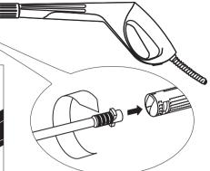
**Step 2** Insert the spray wand of your choice into the wand extension. Push in and turn clockwise to lock spray wand in place.
