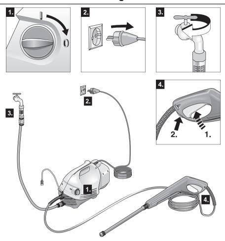
Pull the trigger until there is no more pressure in the appliance, and secure the trigger with the safety ratchet against unintentional opening.
