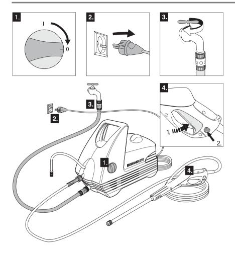
• Pull the trigger until there is no more pressure in the appliance, and secure the trigger with the safety ratchet against unintentional opening.
