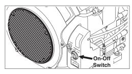
**STEP 2:** Turn engine switch to "OFF" position.
