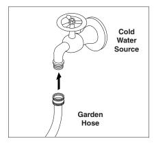
**STEP 3:** Connect garden hose to the cold water source and turn water on completely. Never use hot water.
