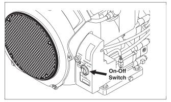
**STEP 6:** Turn the engine switch to "ON" position.
