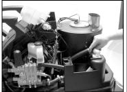
Lift off scale inhibitor reservoir. Remove upper supply hose to water reservoir and route to pump head.
