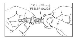
**Note:** Do not blast clean spark plug. Spark plug should be cleaned by scraping or wire brushing and washing with a commercial solvent.
